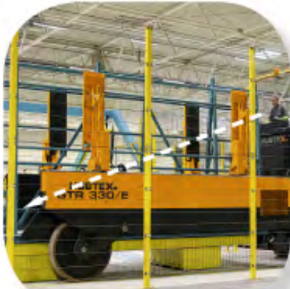
>> liftable operator's platform for best visibility during stillage handling
