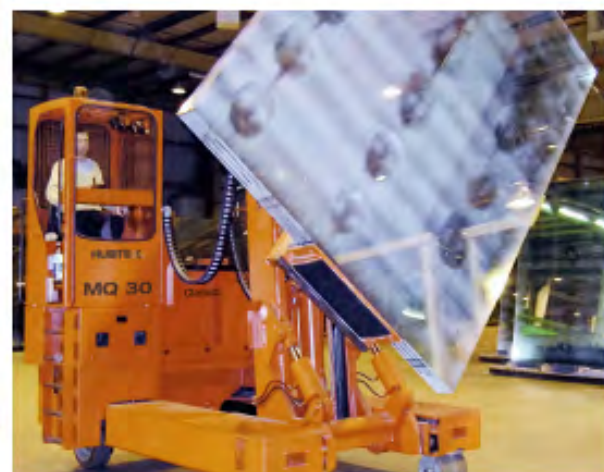
MQ 60 R for rotation of LES-glass packs from portrait to landscape and vice versa
