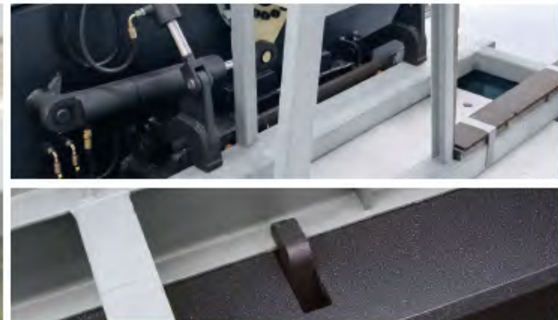
Different versions of glass stillage securing devices to fix the stillage on the platform
