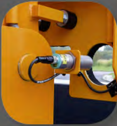
>> sensors on clamps to avoid pressure on glass packs
