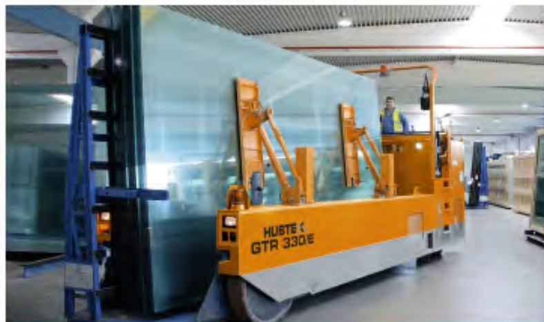
GTR 330 E for indoor transport of L-stillages with 33 tons of glass
