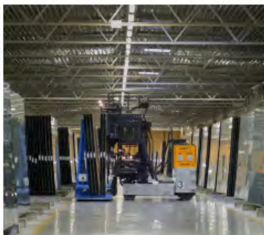
M 150 moves glass packs from a stillage to floor bearers in a narrow aisle
