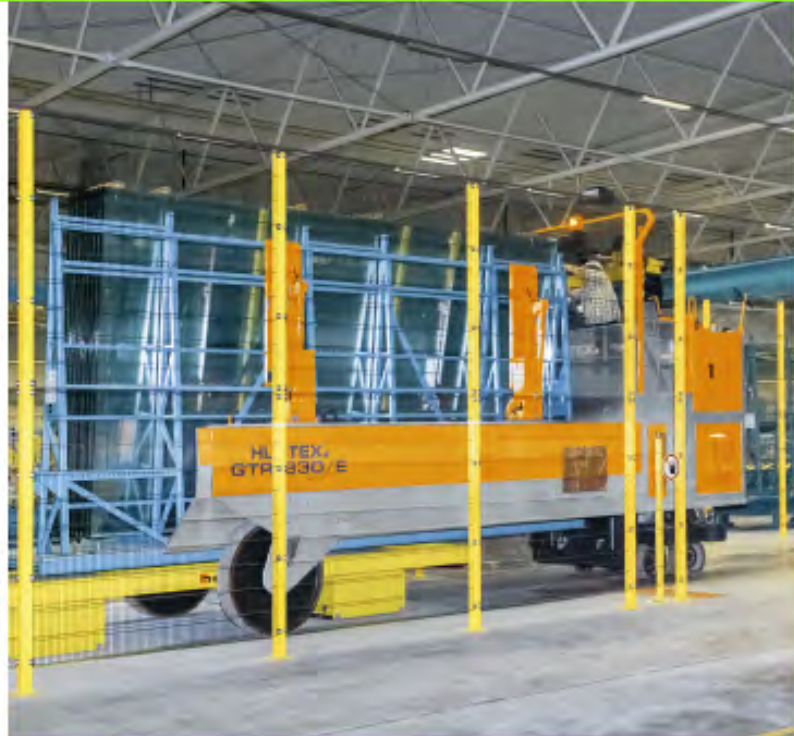
GTR 330 E unloading 33 tons stillage from cold end stacker
