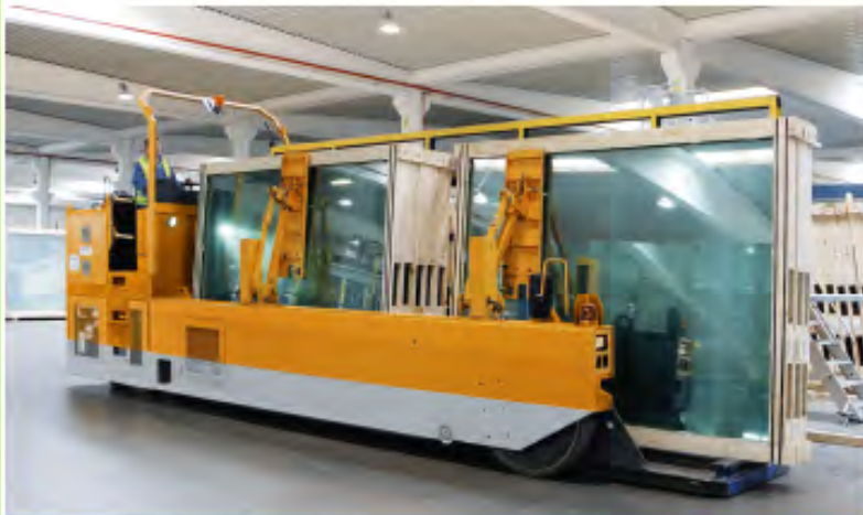
GTR 330 E transporting L-stillage with glass packs in end caps
