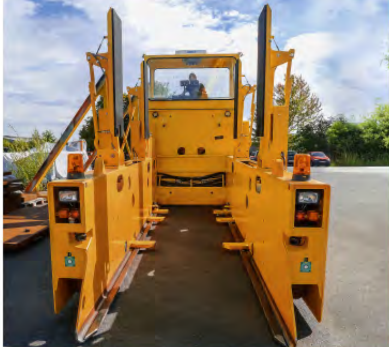
GTR with special device to transport glass stillages with fork pockets
