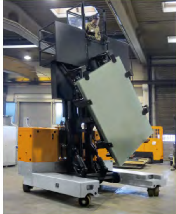
NEW Product: M 40 R (1-man version) for rotation of glass packs to feed a coating line
