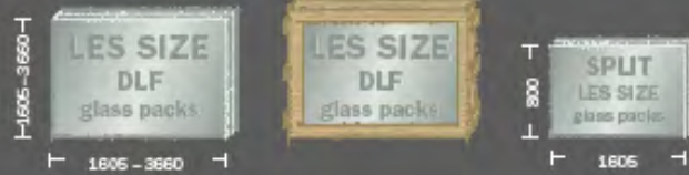
M 90 handling glass packs in end caps
