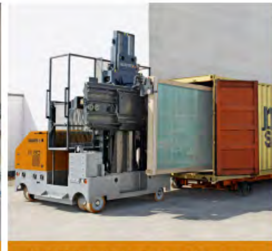
M 80 S0 for loading/unloading of glass in end caps into/out of 20 feet closed sea containers
