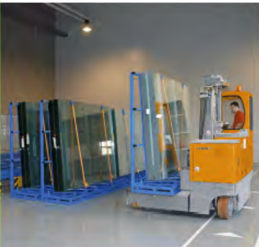
MQ 45 handles L-stillages with raw glass
