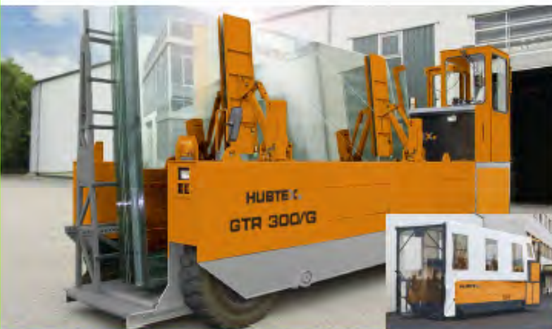
GTR 300 G (LPG) with big-sized rubber tires for combined in- and outdoor use
