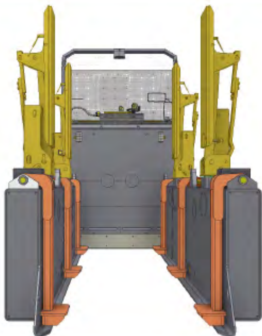
GTR with 180° foldable lifting arms to handle stillages with different widths
