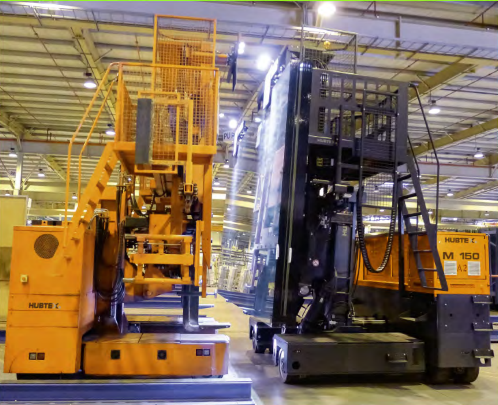
M 150 (year of construction 1996) and M 150 (year of construction 2012) work together during sophisticated glass pack hand-over process to change tin and air side of the glass.
