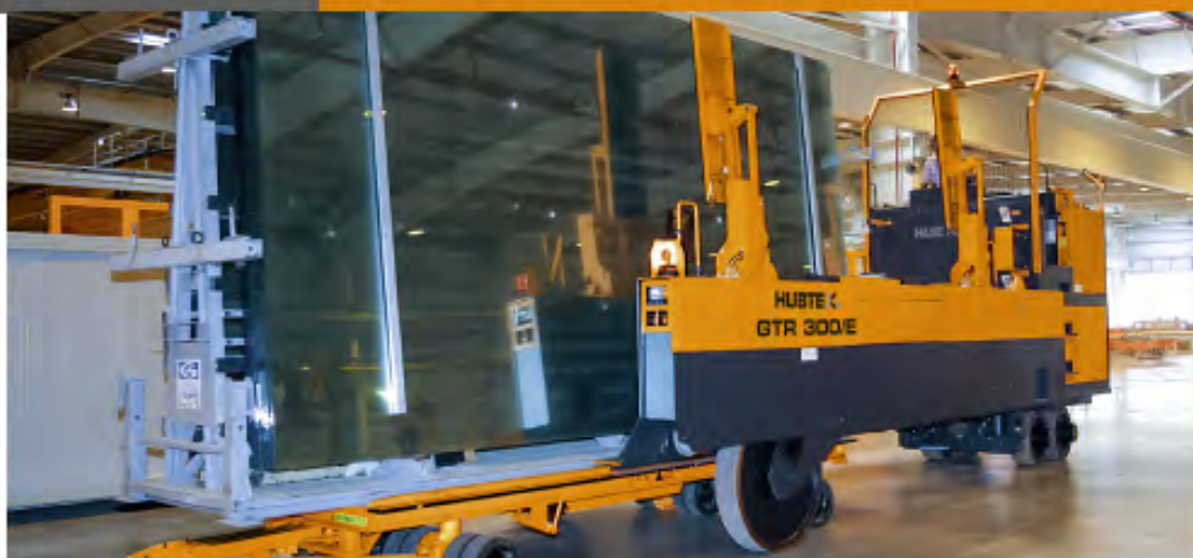
GTR unloading stillage from trolley
