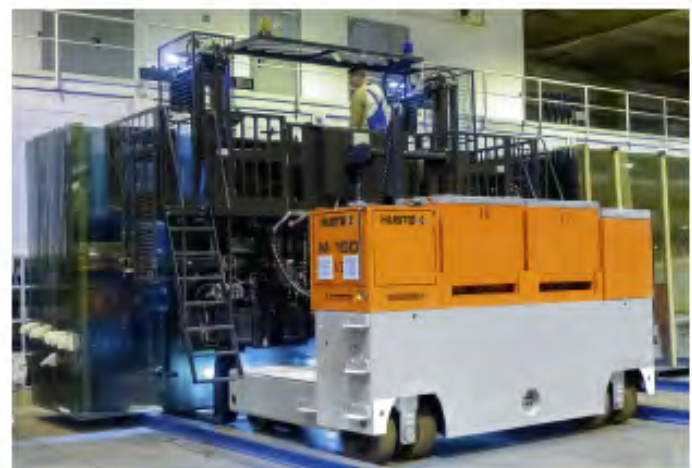
M 150 storing glass packs on floor bearers to increase warehouse density
