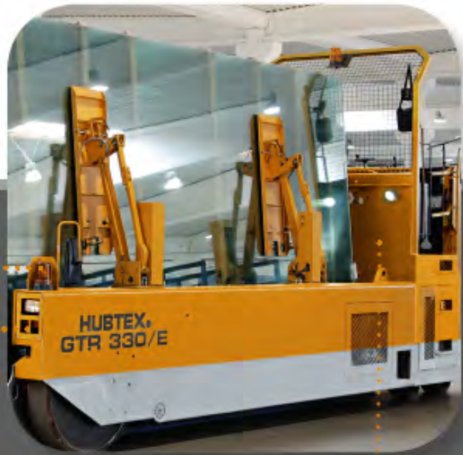
>> glass clamps with increased retention force (curve-drive proof)
