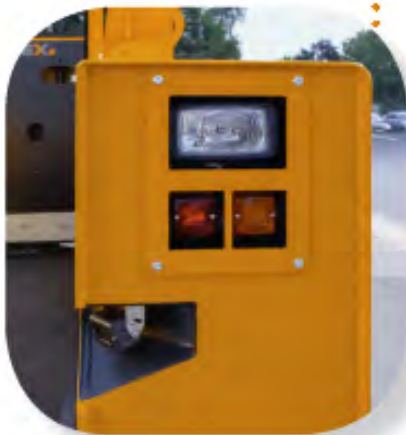
>> frame-integrated color camera and illumination for more safety
