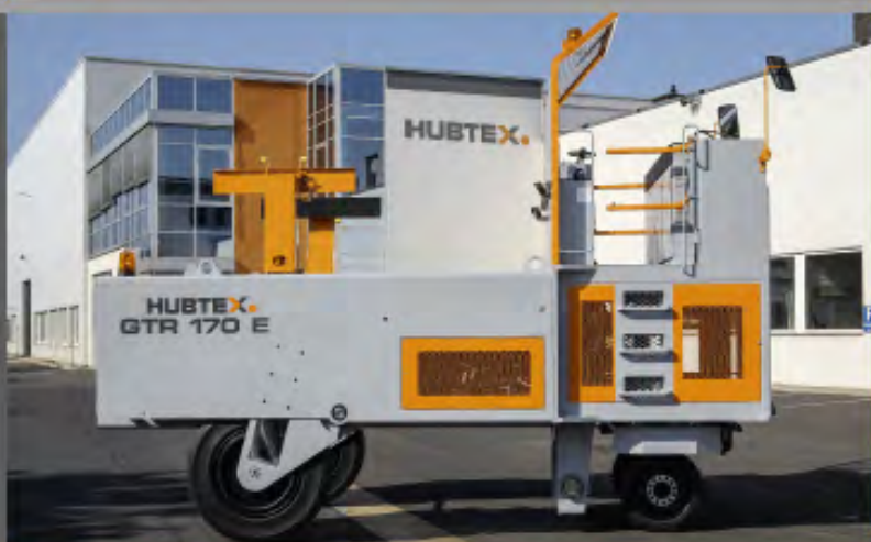
GTR for handling of LES stillages in a coating line
