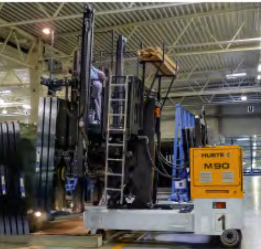
M 90 storing glass packs on floor bearers
