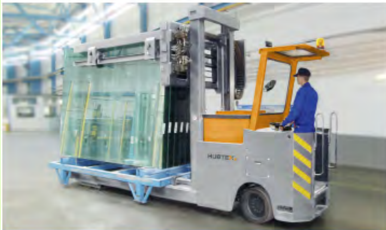
Glass securing device adjustable to different glass pack heights and widths
