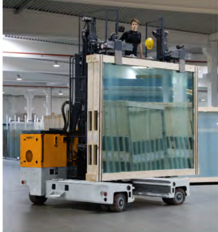
M 90 handling glass packs in end caps
