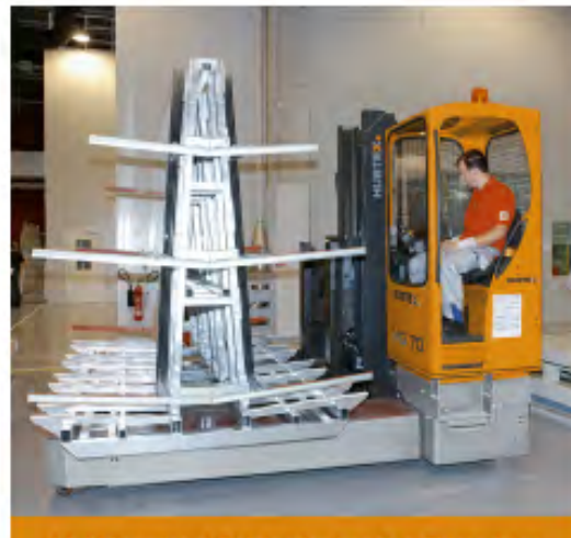
Multidirectional Sideloader handles PV-modules on an A-stillage
