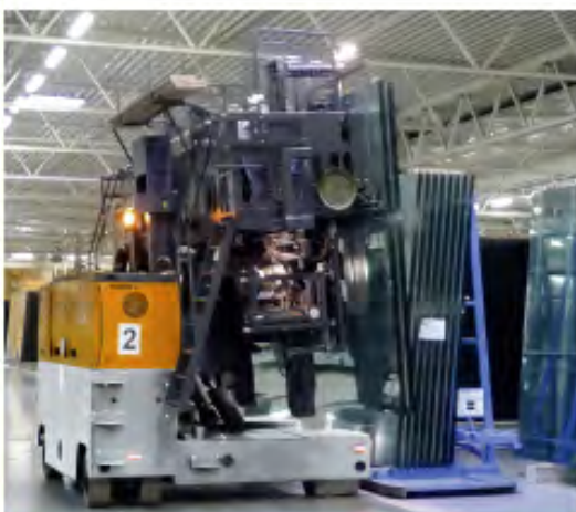
M 150 is able to load/unload a stillage with 30t glass in 2 working cycles
