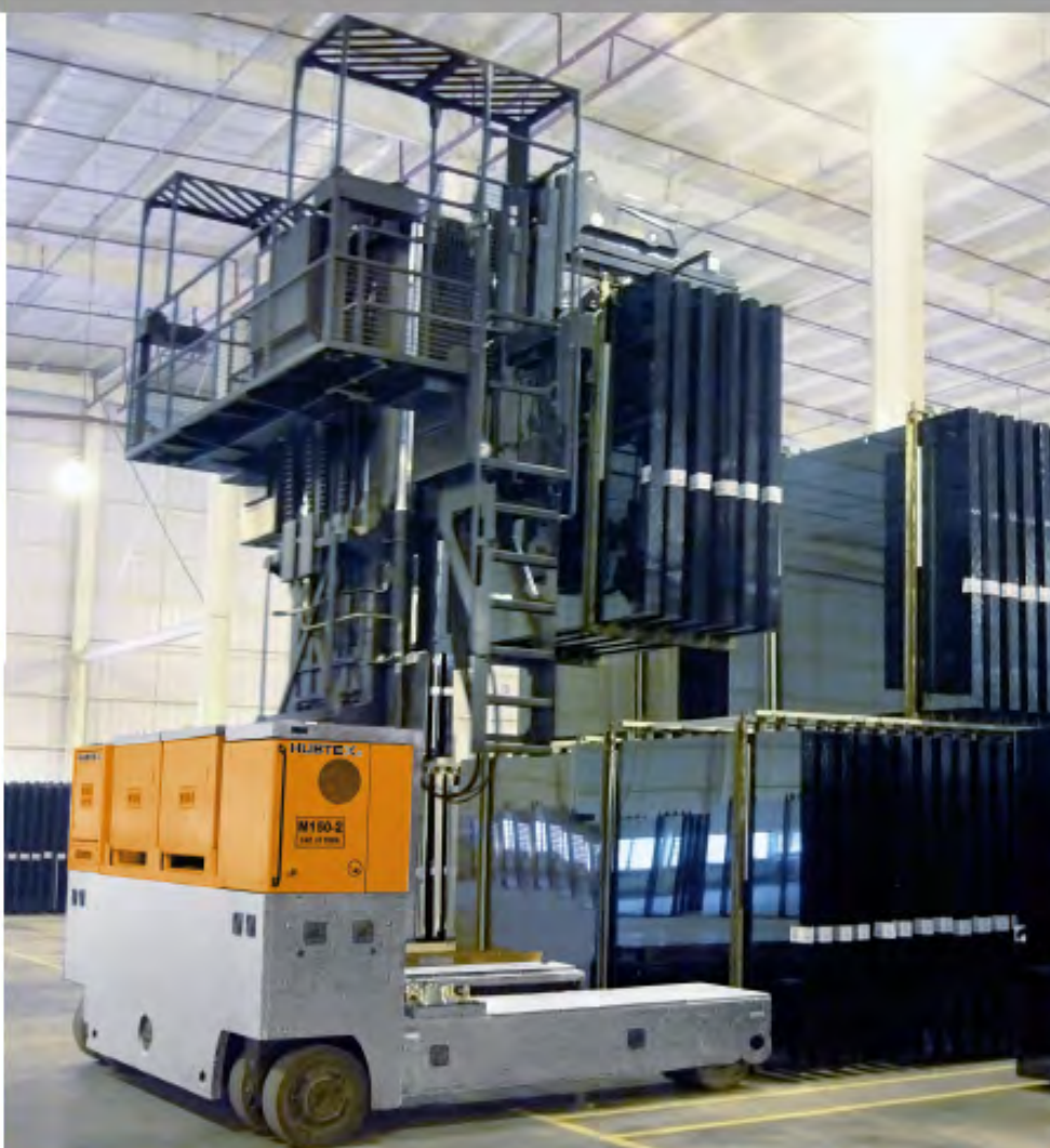
M 150 S0 stores glass packs in collares on two levels
