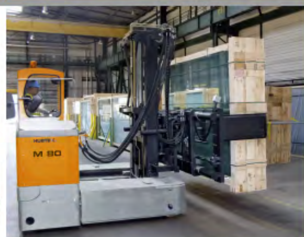
MQ 80 for handling glass packs in wooden crates up to 8 tons
