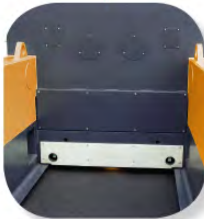
>> sensors for automatic speed reduction during stillage pick-up
