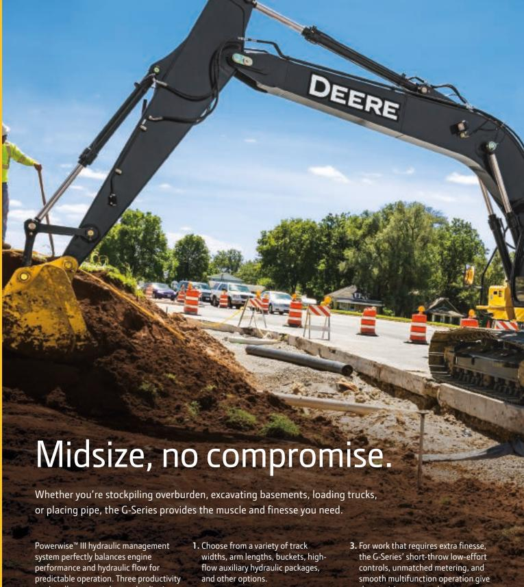
modes allow you to choose the digging style that fits the job. High productivity delivers more power and faster hydraulic response to move more material. Power delivers smooth and balanced metering for normal operation. **Economy** reduces top speed and helps save fuel.
