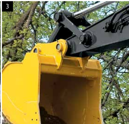
3. Tungsten-carbide coating creates an extremely wear-resistant surface to protect the all-important bucket-to-arm joint.
