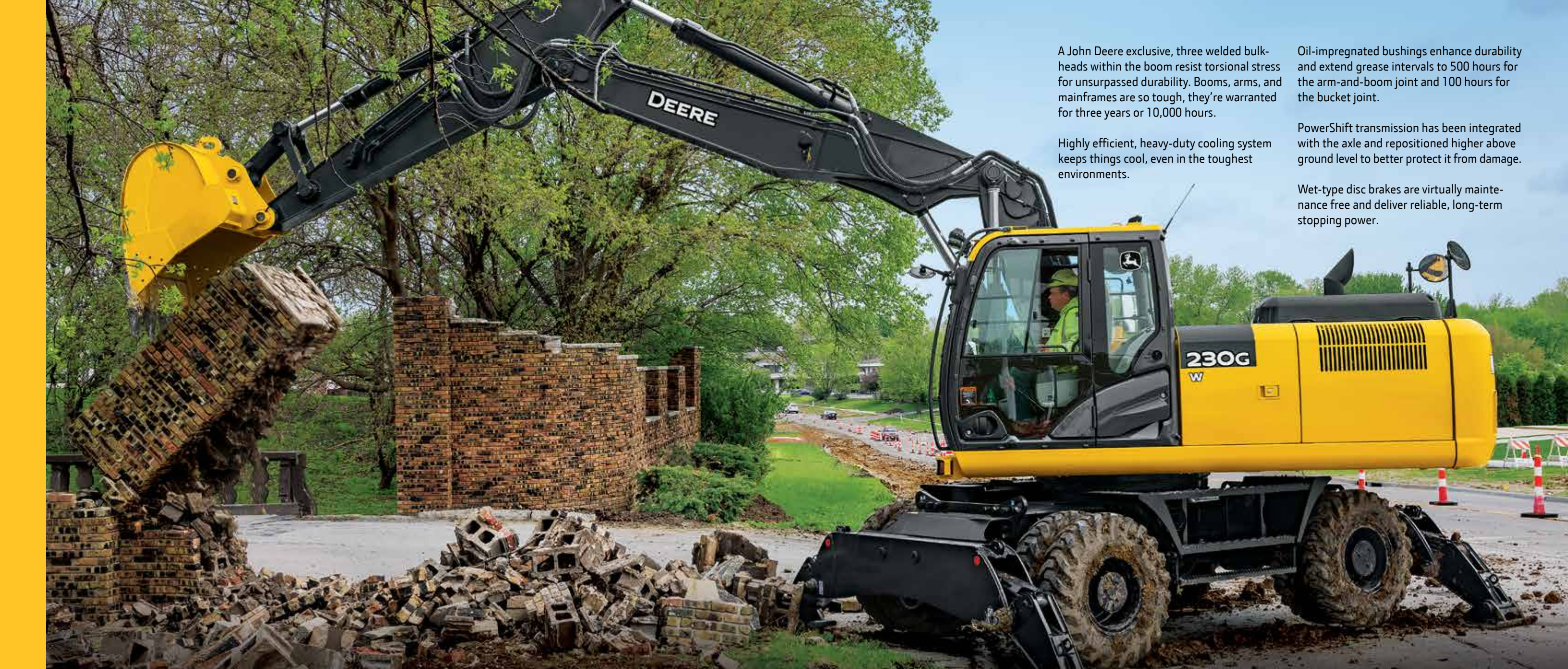
3. Tungsten-carbide coating creates an extremely wear-resistant surface to protect the all-important bucket-to-arm joint.
