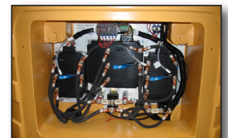
Rear Controller Compartment and Counterweight
